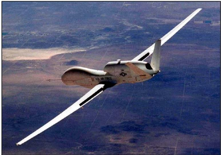
Figure 7: Global Hawk UAV used by the US Air Force for surveillance missions
