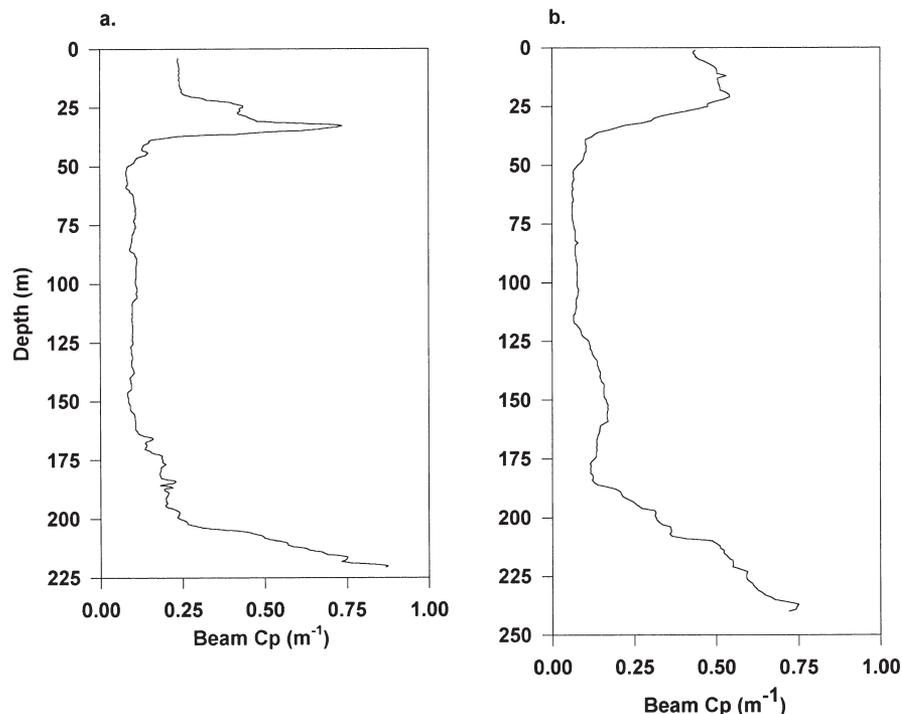
*Figure 2. Particle attenuation ( $c_p$ ) profiles showing bottom nepheloid layers in Wilkinson Basin in August 1995 (a) and Jordan Basin in September 1995 (b) obtained from transmissometer casts ( $c_p$  = total light attenuation minus attenuation due to water and dissolved organic matter).*
